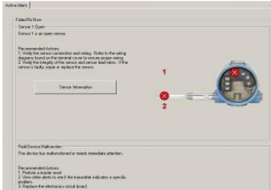
**Fig. 7 - Field Device Malfunction and Recommended Action**
