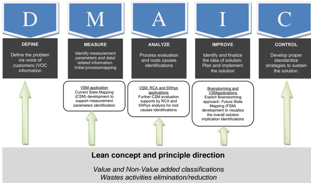
**Fig. 1 – Methodology structure of DMAIC and Lean applications**
