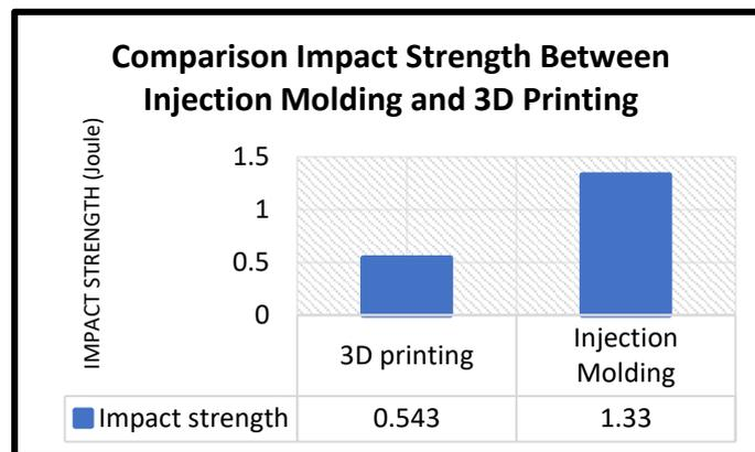
Fig. 4.6 - Comparison of impact strength of PCL/PLA between samples produced using injection molding and 3D printing method.
