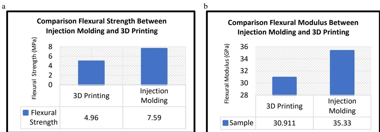
Fig. 4.4 – (a) Flexural strength and (b) Flexural modulus of sample produced using 3D printing and injection molding
