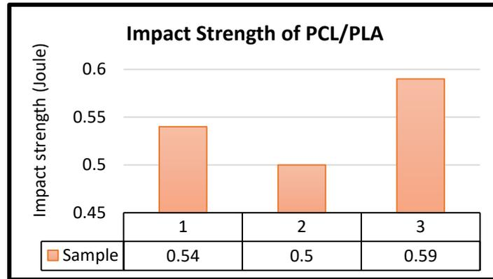
Fig. 4.5 - Impact strength of PCL/PLA sample prepared using 3D printing.
