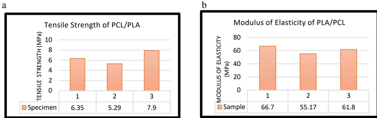
**Fig.4.1 – (a) Tensile strength and (b) Modulus of elasticity of PCL/PLA composites**
