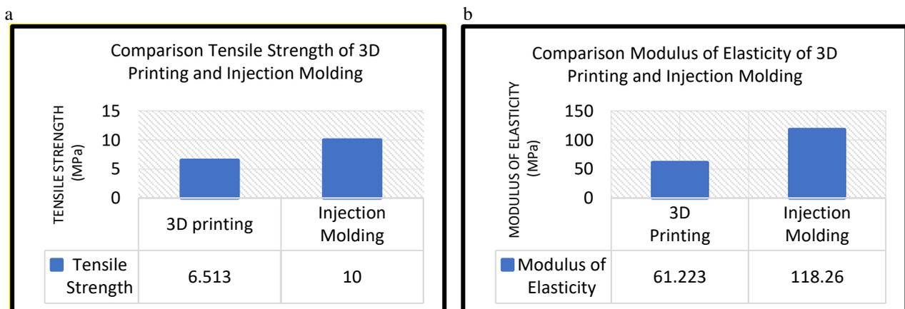
**Fig. 4.2 – (a) Tensile strength and (b) Modulus of Elasticity of sample produced using injection molding and 3D printing**
