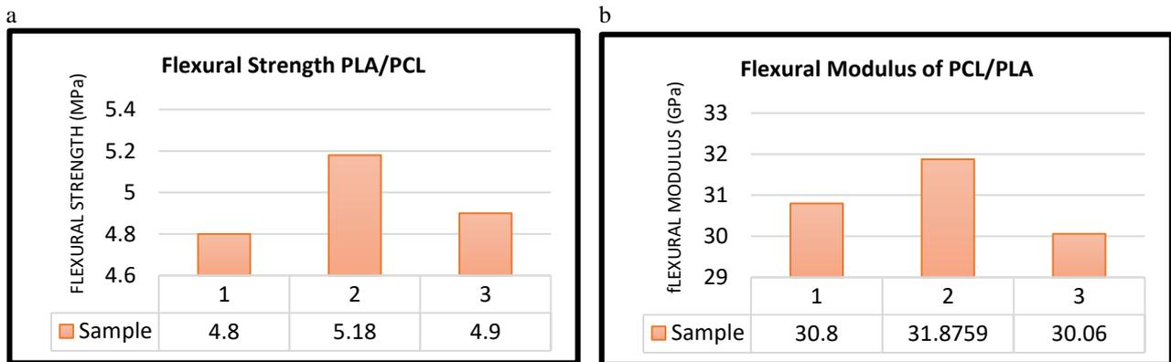
Fig. 4.3 – (a) Flexural Strength and (b) Flexural Modulus of PLA/PCL sample produced by 3D printing.
