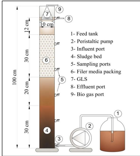
Fig. 1 Schematic diagram of the HUASB reactor.
