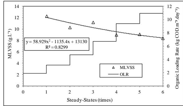
Fig. 4 The development of biomass concentration (for 196 days of operation) in term of MLVSS.
