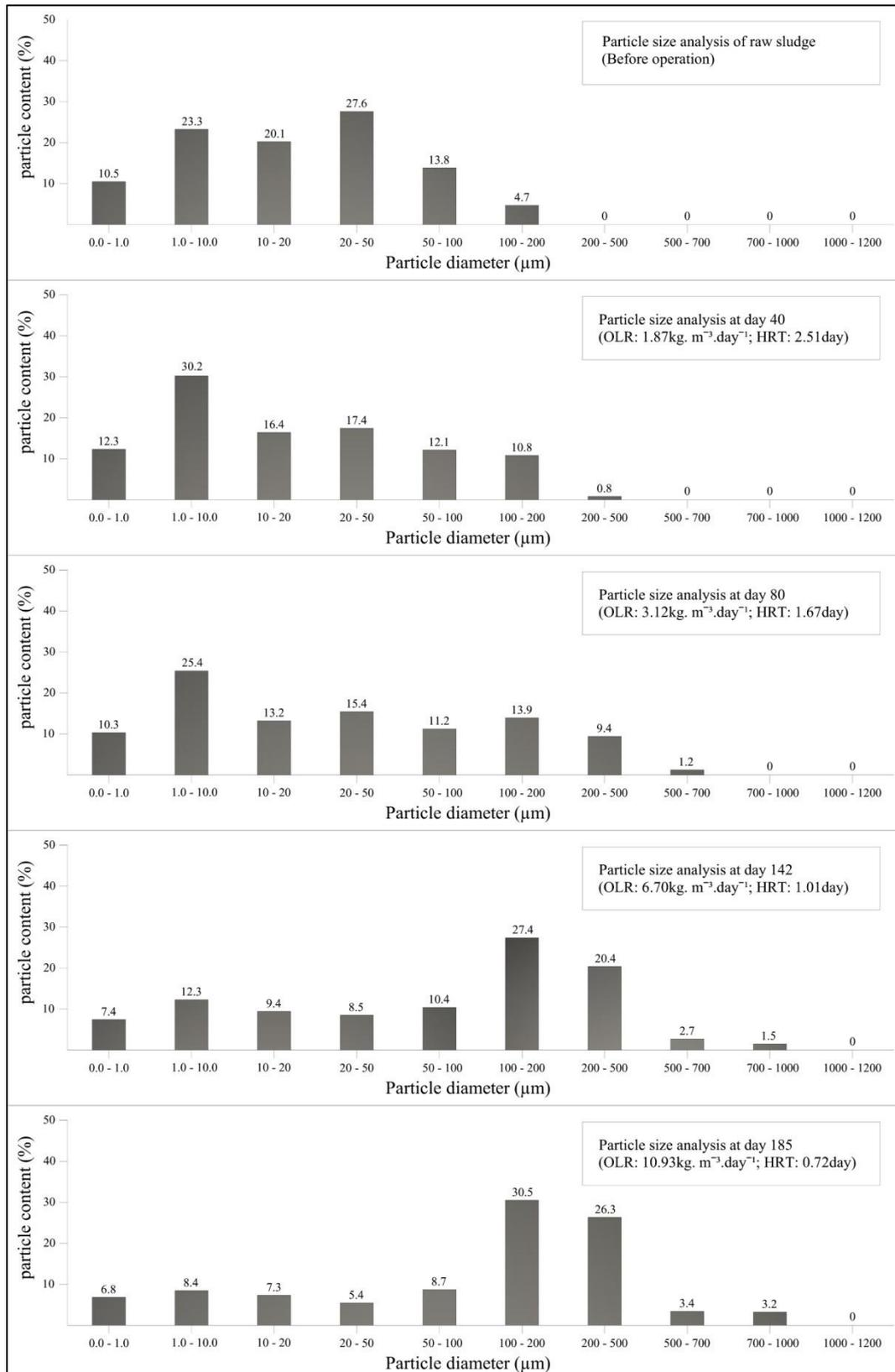
Fig. 2 The particle size distribution for the developed sludge aggregation.
