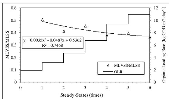
Fig. 6 MLVSS/MLSS Ratio (for 196 days of operation).
