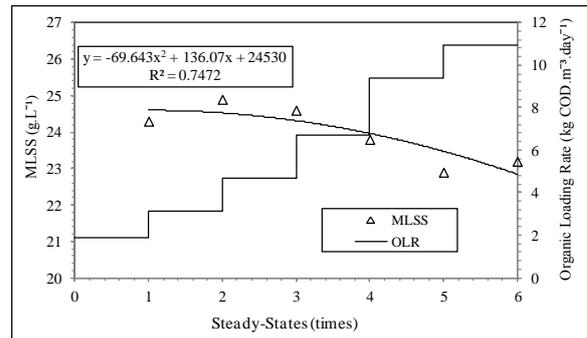
Fig. 5 The development of biomass concentration (for 196 days of operation) in term of MLSS.
