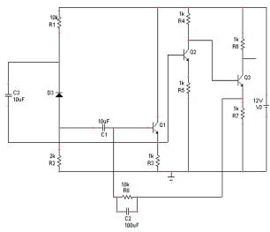
Fig. 6 Bootstrapped transimpedance amplifier circuit
