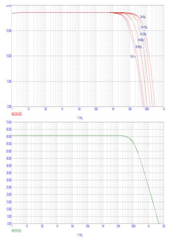
Fig. 12 Frequency response composite transimpedance amplifier
