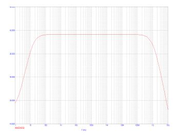
Fig. 8 Frequency response bootstrapped transimpedance amplifier
