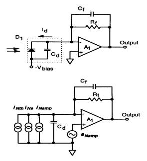
Fig. 4 Transimpedance amplifier circuit and noise model
