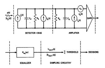
Fig. 5 High impedance amplifier with equalizer
