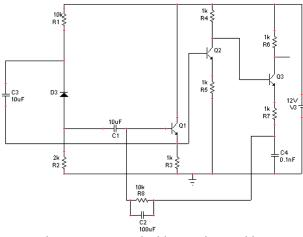
Fig. 7 Bootstrapped with capacitor peaking transimpedance amplifier circuit
