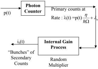
Fig.3 Model of is(t) generation process
