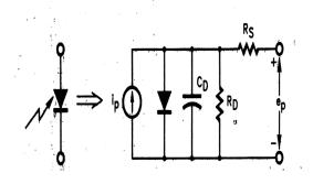
Fig.2 Photodiode circuit model
