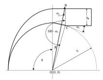
Fig 2. The nozzle roof curvature radius
