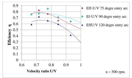
Fig. 8. Efficiency vs Velocity ratio
