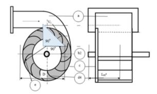
a = nozzle, b = shaft, c = disk, d = blade, e = water jet
