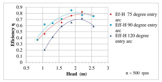
Fig. 7. The Efficiency vs the Head
