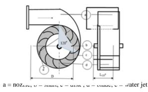
Fig. 3c. Turbine model with nozzle entry arc of 120°
