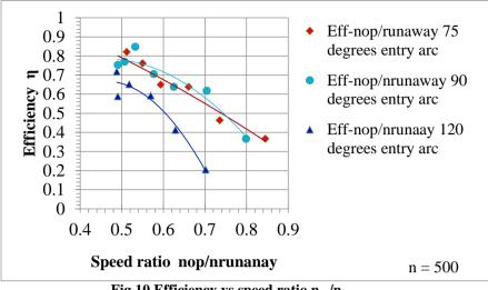
Fig.10 Efficiency vs speed ratio nop/nrunaway
