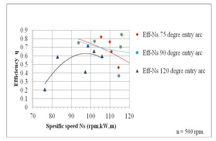
Fig. 9. Efficiency vs Specific speed
