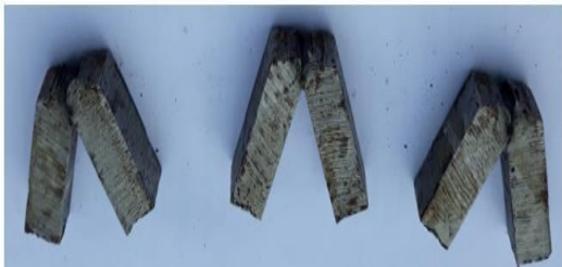
Fig. 7 - Non-welded Heat treated (NWHT) After Impact
