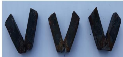
Fig.6. -Welded-Non-heat Treated (WNHT) After Impact
