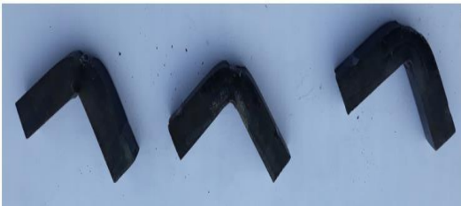
Fig. 5 - Welded-Heat treated (WHT) After Impact
