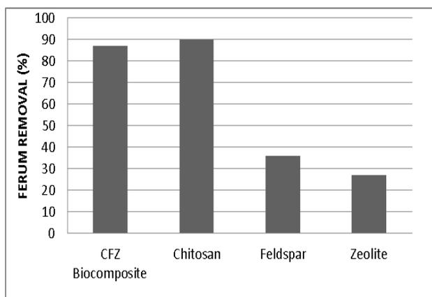
Figure 4 Comparison on ferum removal between media
