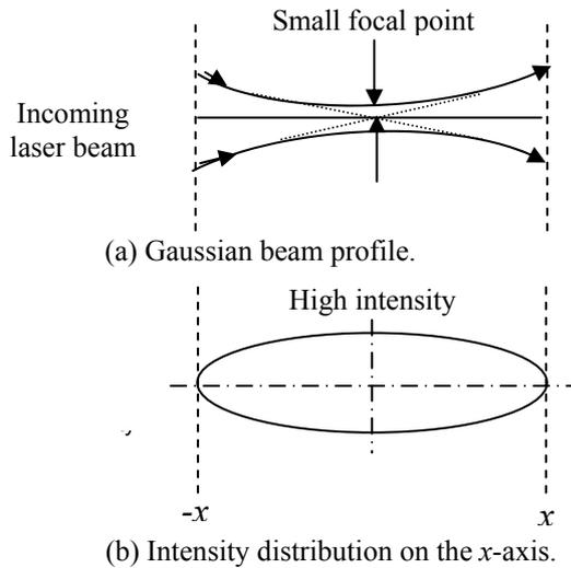
Fig. 4 The distribution of plasma beam along the  $x$ -axis.
