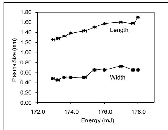
Fig. 6 The size of laser plasma as a function of laser energy.
