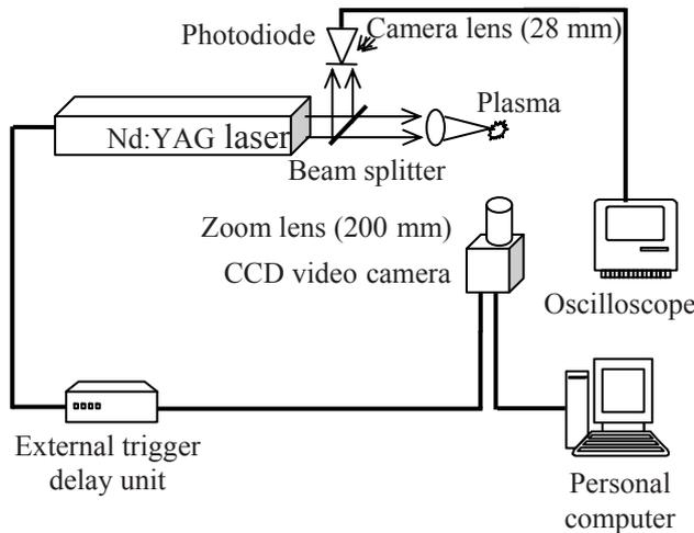
Fig. 1 Experimental setup to diagnose the laser plasma by using high-speed photographic technique and interface with image processing system.
