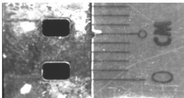
Fig. 2 Used film and millimeter ruler for magnification calibration process.
