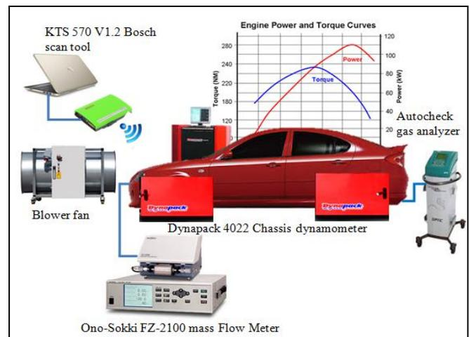
Fig. 2 Schematic diagram arrangement of engine test condition
