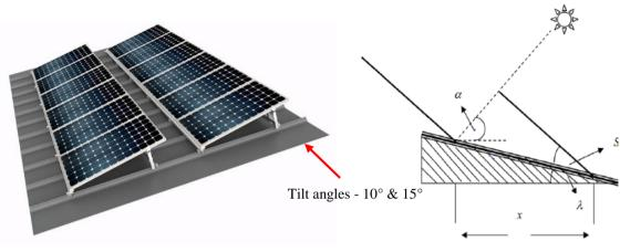
Fig. 3 – (a) Cross Section; (b) Tilt Angles
