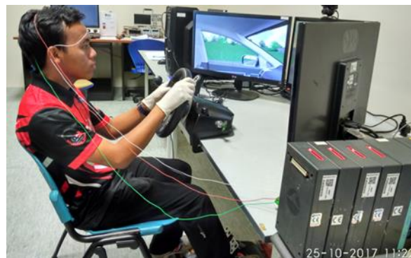
Fig. 3 – Experiment setup using driving simulator and EEG in laboratory
