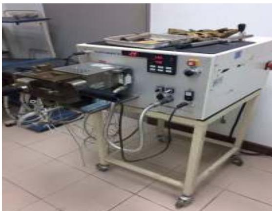
Fig 1 Barbender machine use to mix the composition
