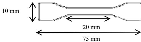
Fig 4 Dog bone sample for tensile testing [7]
