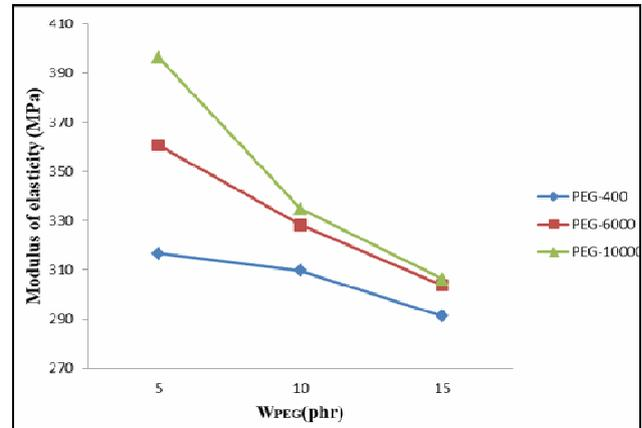
Fig 8 Effect of PEG content on modulus of elasticity of PCL/PLA/PEG blends
