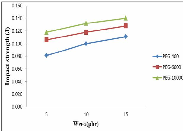
Fig 9 Effect of PEG content on impact strength of PCL/PLA/PEG blends.
