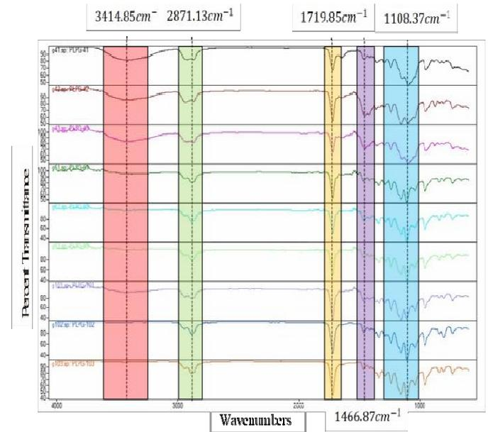
Fig 6 FTIR of PCL/PLA/PEG with different content and molecular weight.
