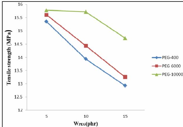
Fig 7 Effect of PEG400, PEG6000 and PEG10000 content on tensile strength of PCL/PLA/PEG blends.
