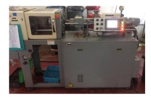
Fig 2 Injection molding machine used to produce samples
