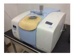
Fig 3 Fourier transform infrared spectroscopy (FTIR) machine
