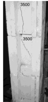
Fig.5 Experimental failure mechanism [10]
