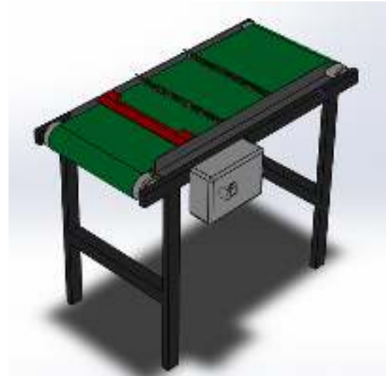
Fig. 2 The design of coated peanut separator machine that consists 3 parts of separator section and PVC conveyor belt.
