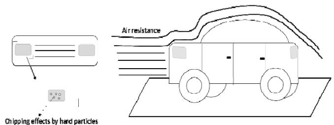
Fig. 4 Schematic drawing of head lights exposed to erosion
