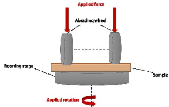
Fig. 15 Schematic drawing of a Taber Abraser tribometer.
