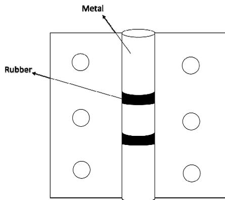
Fig. 1 Hinge for sliding applications of a door
