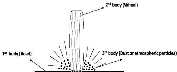
Fig. 5 Schematic drawing of a wheel and a road in contact with an introduction of dust or atmospheric particles as 3<sup>rd</sup> body (2 & 3 bodies friction)
