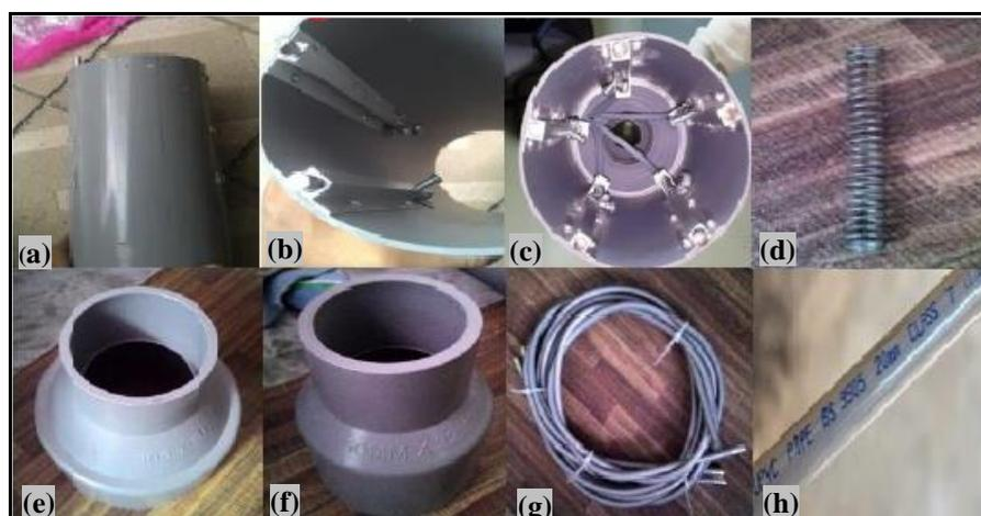
**Fig. 4- Components and Fabrication steps. (a) PVC pipe cutting for casing; (b) door latch installation as jaws; (c) complete latch installation; (d) compression spring installation; (e) reducer installation; (f) pipe PVC connector; (h) connecting jaws and pedal using cable; (g) Installation of pole**
