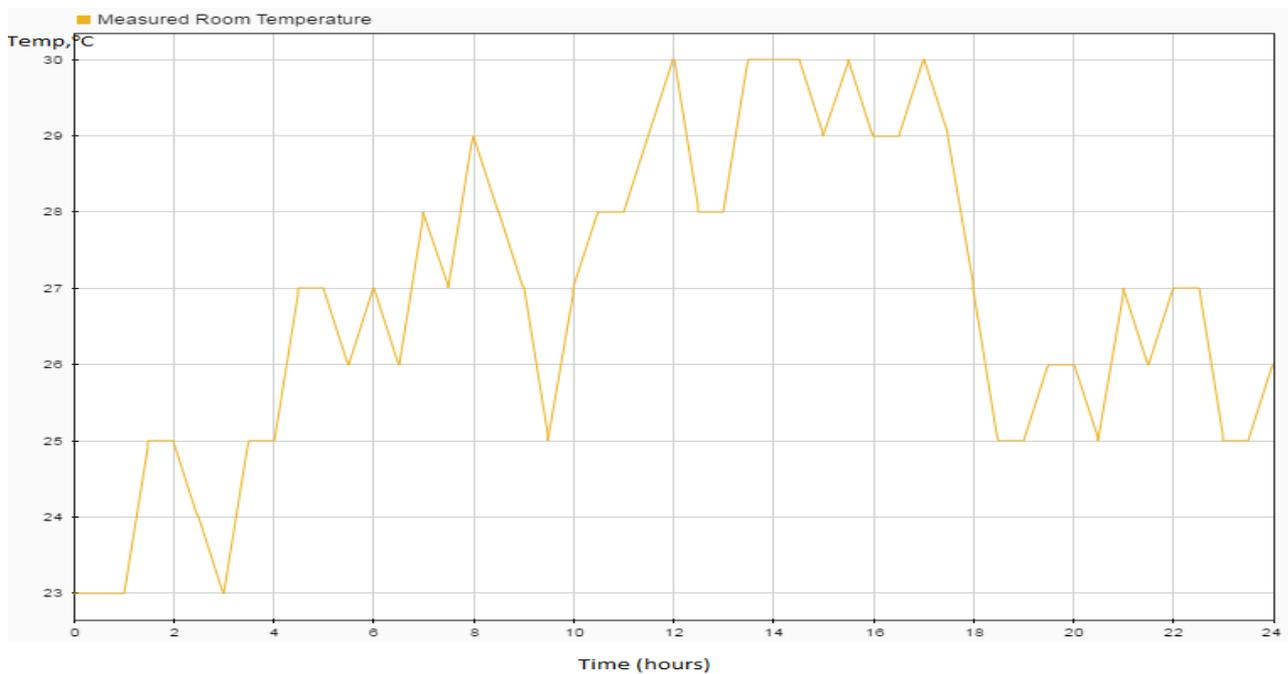
**Fig. 9 – Room temperature profile without controller (cloudy day)**
