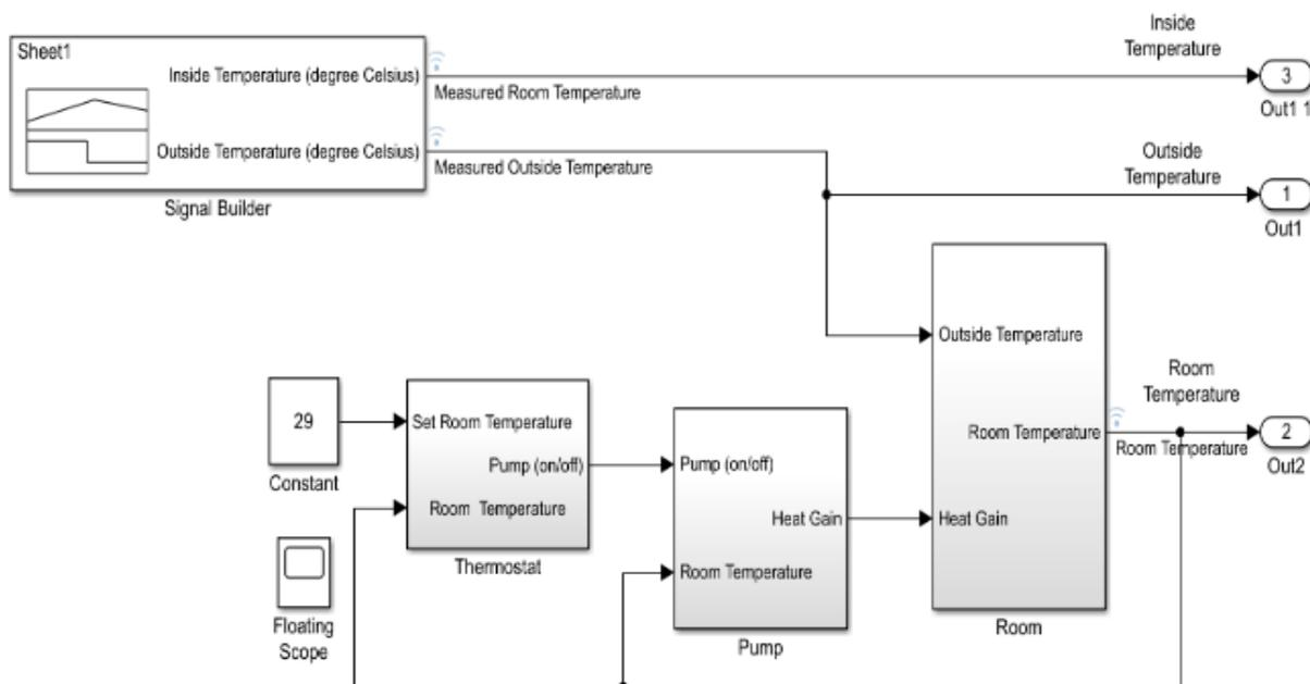
Fig. 4 – Temperature control subsystem
