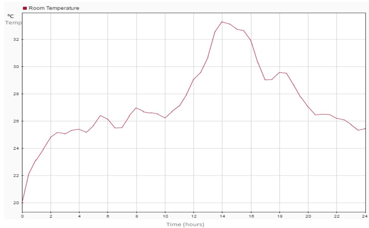
Fig. 7 – Room temperature profile with controller (hot day)
