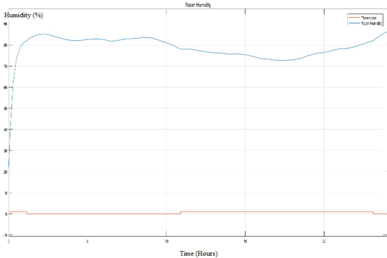
**Fig. 12 –Room humidity profile with controller (hot day)**
