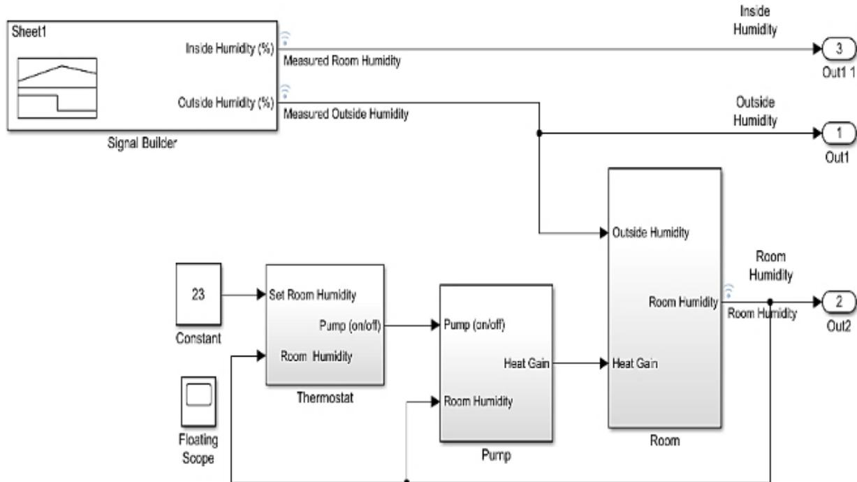
Fig. 5 – Humidity control subsystem
