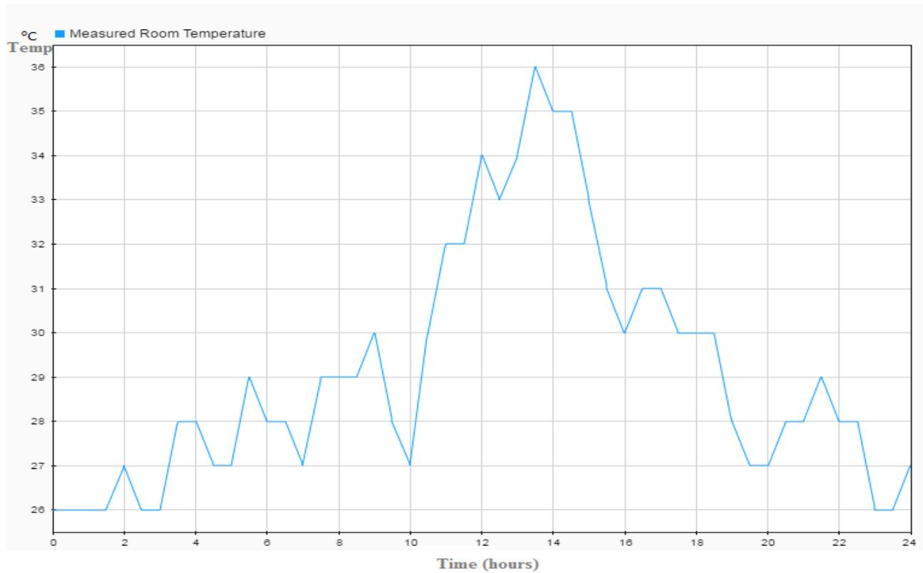
Fig. 6 – Room temperature profile without controller (hot day)
