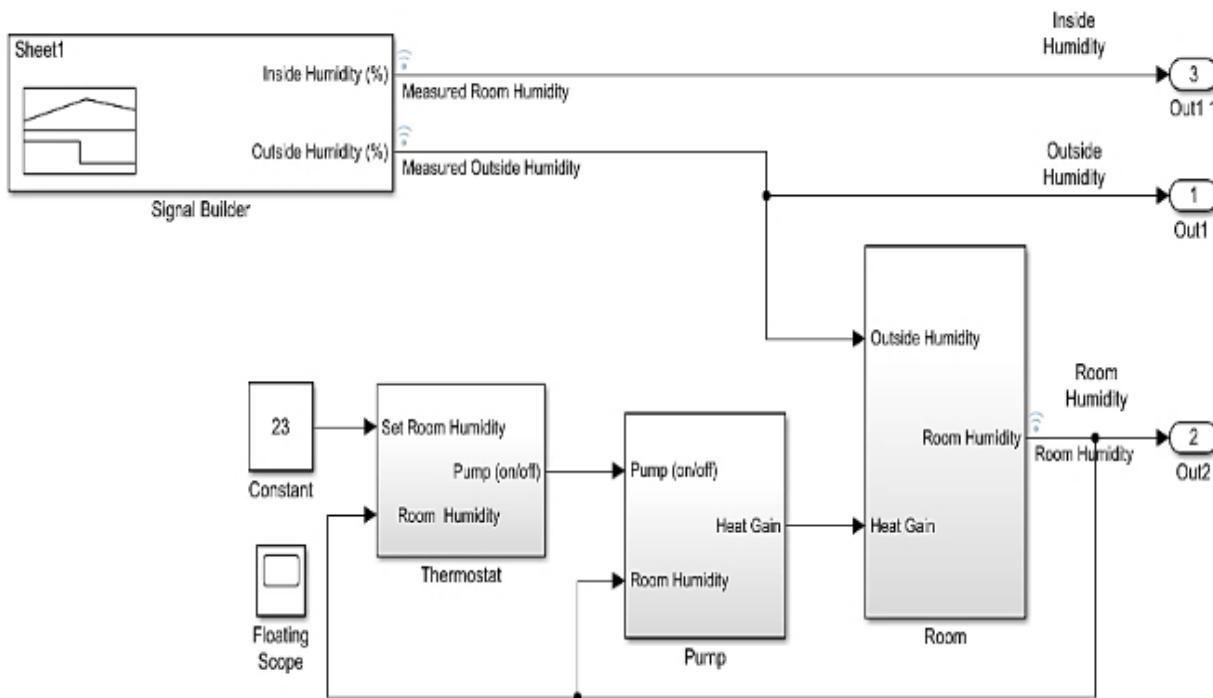
**Fig. 5 – Humidity control subsystem**
