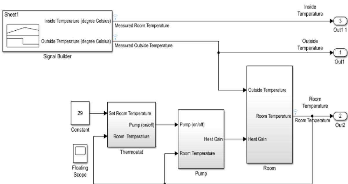
Fig. 4 – Temperature control subsystem
