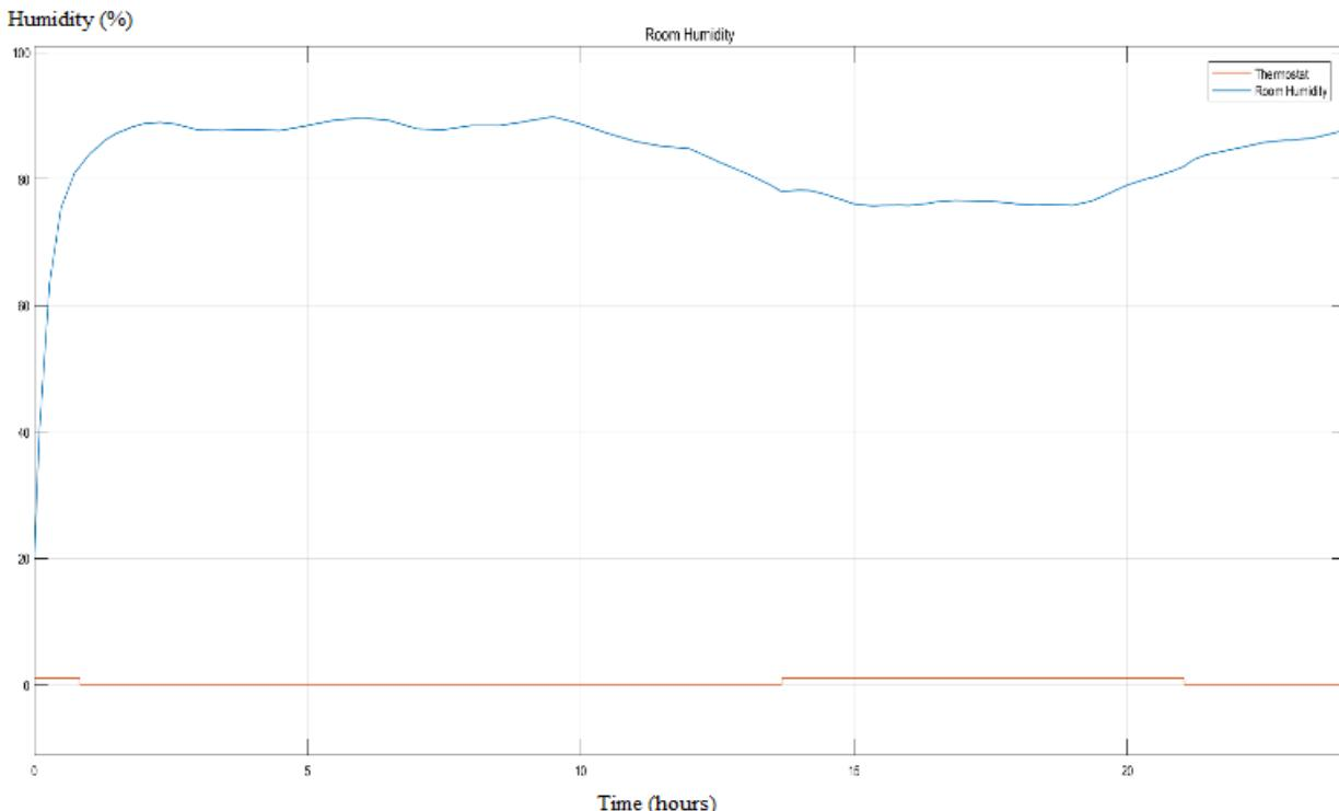
Fig. 14 –Room humidity profile with controller (cloudy day)
