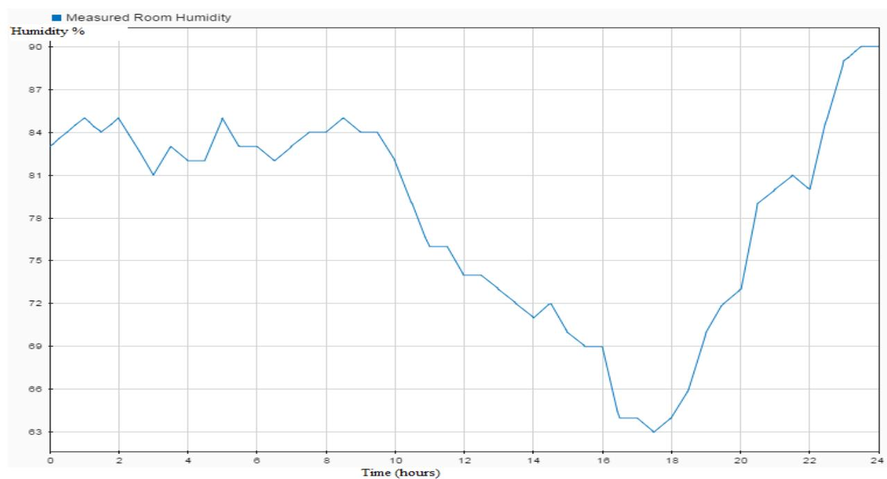
**Fig. 11 –Room humidity profile without controller (hot day)**
