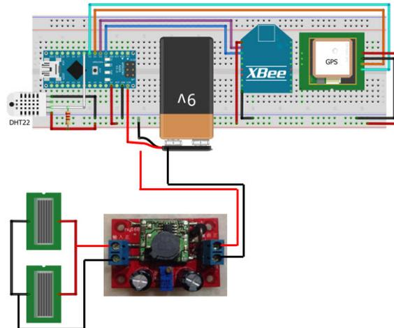
Fig. 3 - Schematic of the environmental monitoring part
