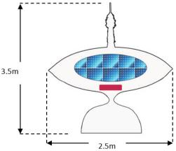
Fig. 2 - Schematic of the design of the proposed Solar-kite equipped with thin solar cells and electronics
