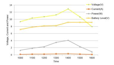
Fig. 6 - Output Voltage, Current and Power at different times of a typical day
