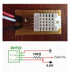
Fig. 4 - Schematic and actual circuit of DHT22 sensor module
