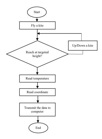
Fig. 1 - The overall process flow of a solar-kite for environmental monitoring
