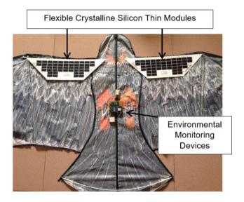
Fig. 5 - A kite prototype (similar) with solar power module and electronic devices
