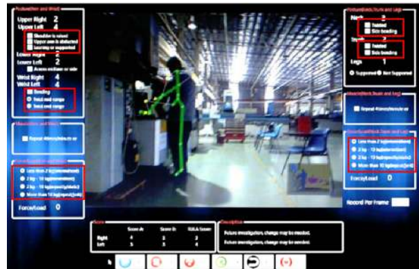
Fig. 3 GUI two - RULA input data and real time results
