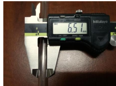
Fig. 3. Diameter values for transparent rod using Vernier caliper
