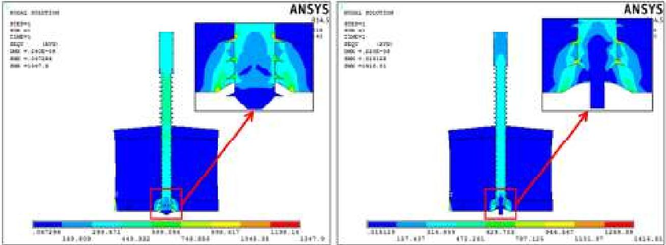
Fig. 3 (a) Highest stress of TC half-pin for titanium alloy (b) Highest stress of TTT half-pin for titanium alloy
