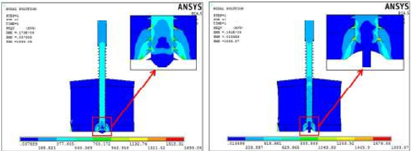
Fig. 4 (a) Highest stress of TC half-pin for stainless steel (b) Highest stress of TTC half-pin for stainless steel
