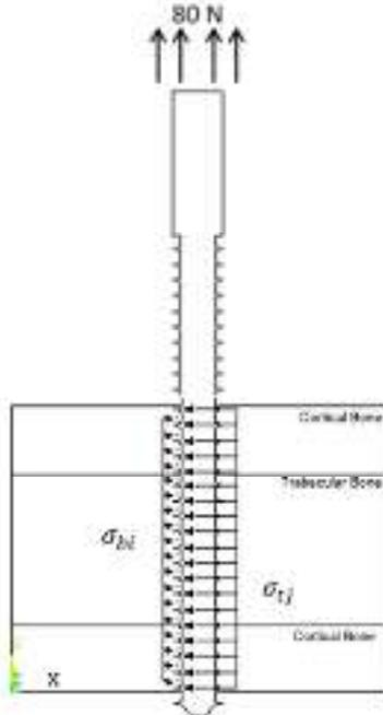
Fig. 1 Boundary condition of two dimensional pin-bone interaction
