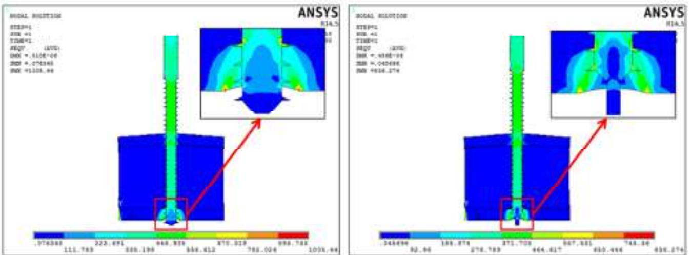
Fig. 5 (a) Highest stress of TC half-pin for magnesium alloy (b) Highest stress of TTC half-pin for magnesium alloy
