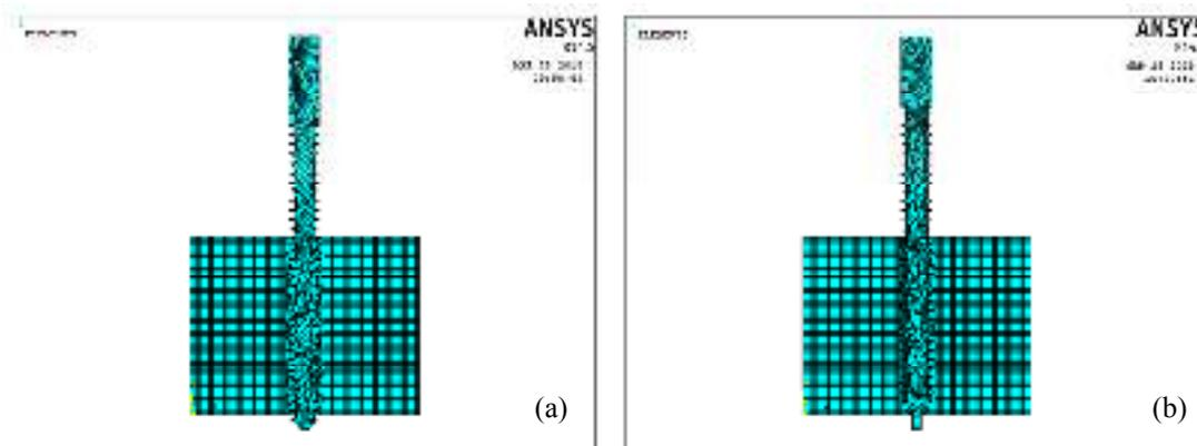
Fig. 2 (a) Meshing of tapered conical half-pin (b) Meshing of trocar-tip tapered half-pin
