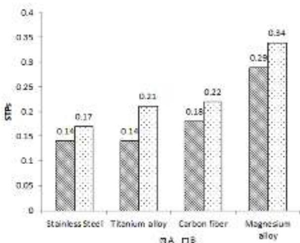
Fig. 7 Effect of pins materials on average STPs
