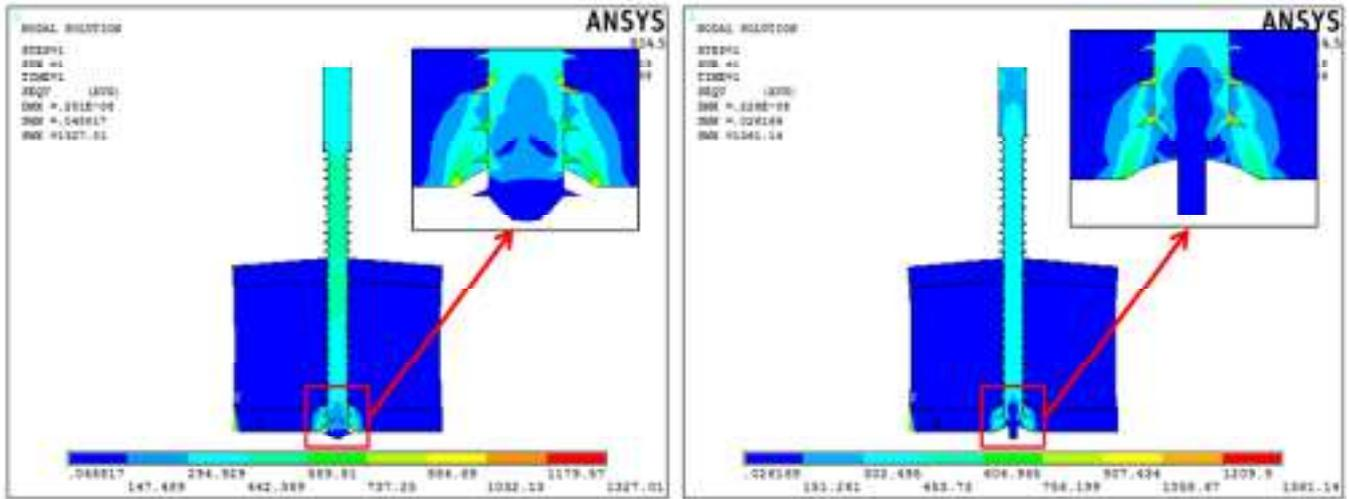
Fig 6 (a) Highest stress of TC half-pin for carbon fiber (b) Highest stress of TTT half-pin for carbon fiber.
