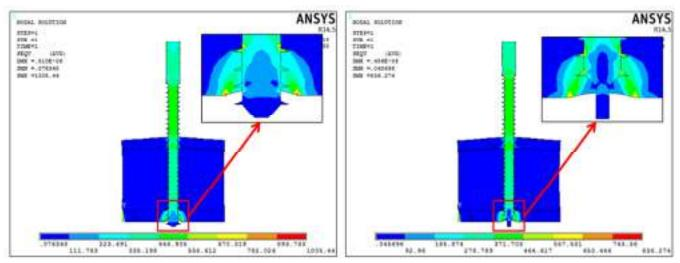
Fig. 5 (a) Highest stress of TC half-pin for magnesium alloy (b) Highest stress of TTC half-pin for magnesium alloy
