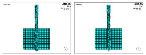
Fig. 2 (a) Meshing of tapered conical half-pin (b) Meshing of trocar-tip tapered half-pin
