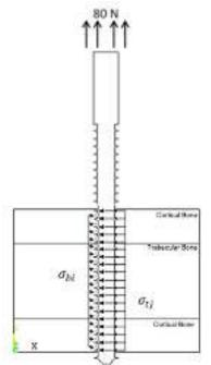
Fig. 1 Boundary condition of two dimensional pin-bone interaction
