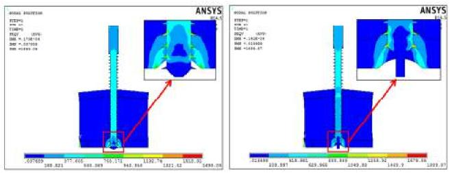
Fig. 4 (a) Highest stress of TC half-pin for stainless steel (b) Highest stress of TTC half-pin for stainless steel
