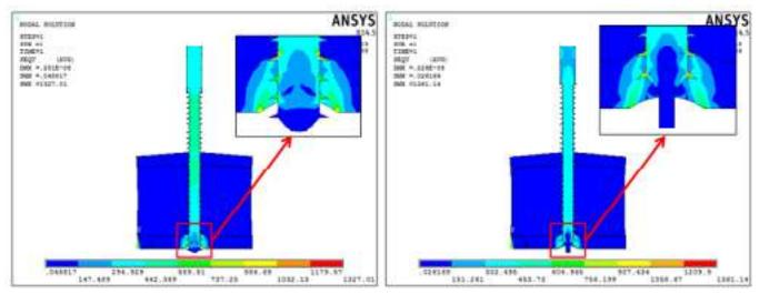
Fig 6 (a) Highest stress of TC half-pin for carbon fiber (b) Highest stress of TTT half-pin for carbon fiber.
