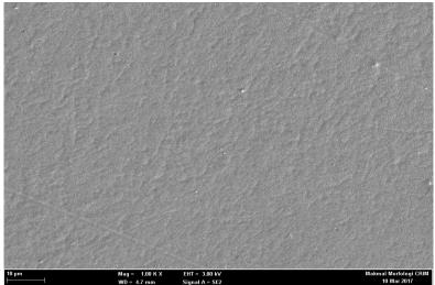
Fig 1 - FESEM micrograph shows surface morphology of P(VDF-TrFE) film of piezoelectric sensor
