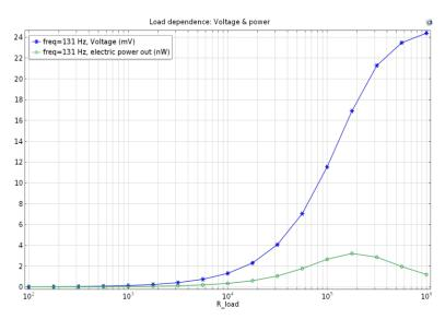
Fig 6 - Electrical properties : voltage and power output with respect to load resistance
