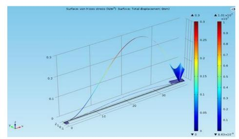
Fig 4 - Mechanical properties: Resonant frequency for displacement and von Mises stress contour
