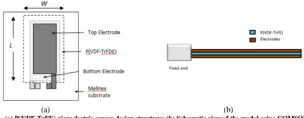
Fig 2 - (a) P(VDF-TrFE) piezoelectric sensor design structure; (b) Schematic view of the model using COMSOL Multiphyics
