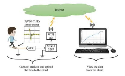
Fig 8 - P(VDF-TrFE) Piezoelectric sensor in IoT application
