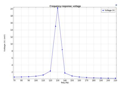
Fig 5 - Electrical properties: Voltage output at resonance frequency
