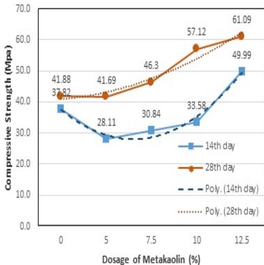
Fig 2. Compressive strength with variation of meta-kaolin addition
