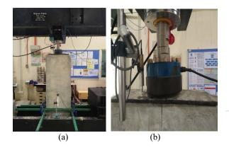
Fig. 5 Axial Load Test. (a) General set up. (b) Load cell and LVDT to capture data.
