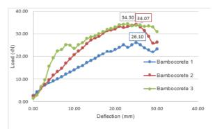
Fig. 8 Flexural bending test on bamboocrete panel
