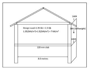
Fig. 4 Load distribution on wall panel
