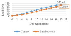
Fig. 7 Axial load test on control and bamboocrete panel
