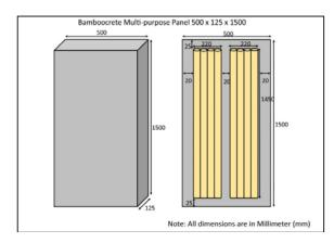
Fig. 1 Bamboocrete Multi-purpose Panel
