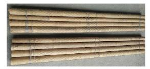
Fig. 2 Bamboo wrapped with wire mesh.
