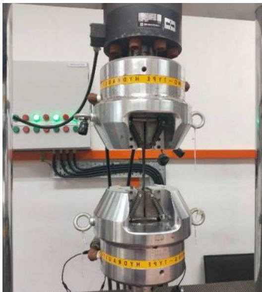
Fig. 5 Tensile testing of Polypropylene-based composite samples
