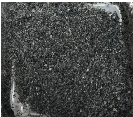
Fig. 3 Composites after the crushing process
