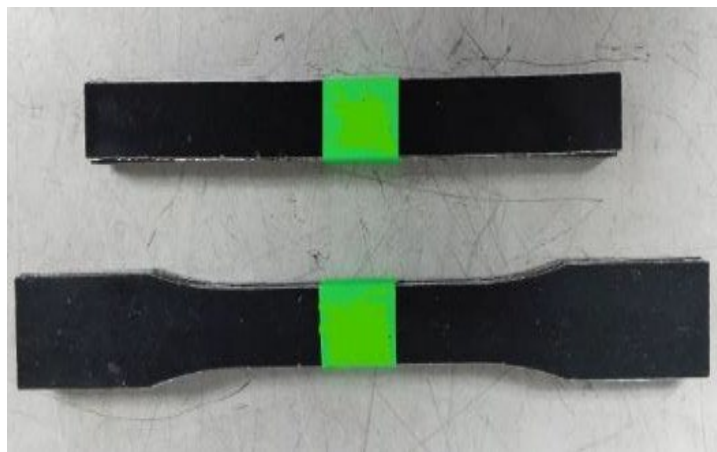
Fig. 4 Hot-pressed Polypropylene composite samples
