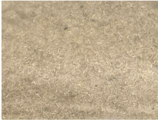
Fig. 1 Bamboo fibers after the sieving process
