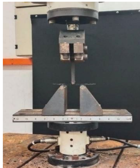
Fig. 6 Flexural testing of Polypropylene-based composite samples
