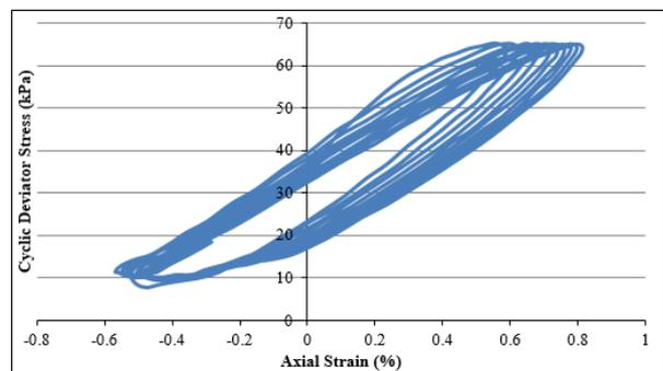
Fig. 2 Hysteresis Loop Results from Cyclic Triaxial Test
