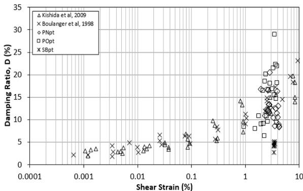
Fig. 9 Correlations of Damping Ratio versus Shear Strain
