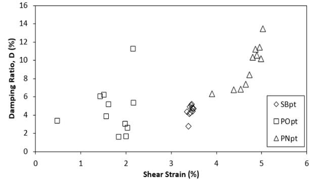
Fig. 5 Relationships between Damping Ratio and Shear Strain for PNpt, POpt and SBpt.
