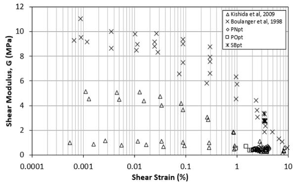
Fig. 10 Correlations of Shear Modulus versus Shear Strain
