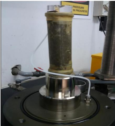
Fig. 1 Sample Setup for Cyclic Triaxial Test
