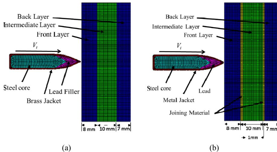
Fig. 3 Finite element model of projectile and laminated plate for: (a) Laminated panel without joining material, (b) Laminated panel with joining materials.
