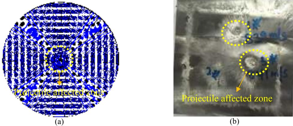
Fig. 4 Comparison of triple-layered plate after the: (a) simulation, (b) ballistic test.
