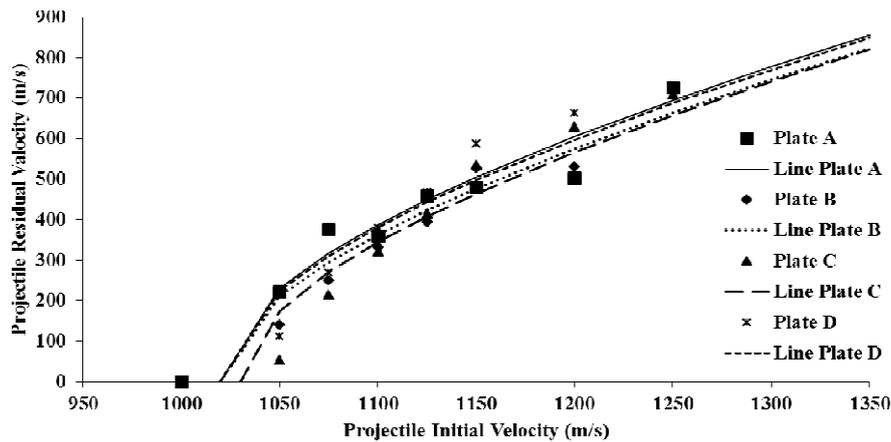
Fig. 7 Predicted residual velocity using the Recht-Ipson model.
