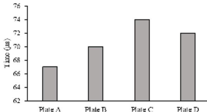
Fig. 6 Comparison of end of penetration for panels subjected to an impact velocity of 900 m/s.
