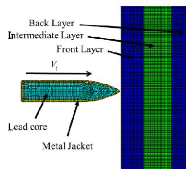
Fig. 2 FE model of panel subjected to 7.62-mm FMJ projectile for validation of FE model.
