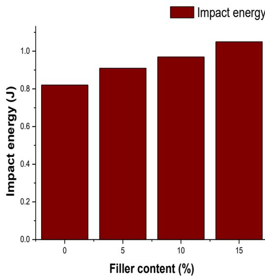
Fig. 7 - Impact energy of composite samples
