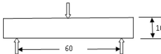
**Fig. 3 - Composite sample for Flexural test**
