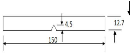
**Fig. 4 - Composite sample for Impact test**
