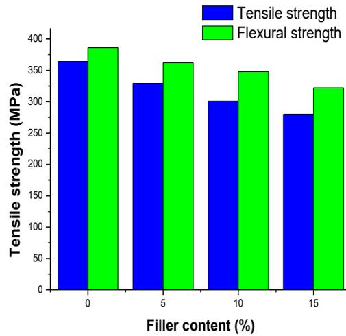
Fig. 6 - Tensile strength and Flexural strength of composite samples
