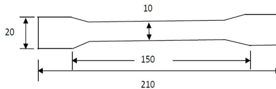
**Fig. 2 - Composite sample for tensile test**
