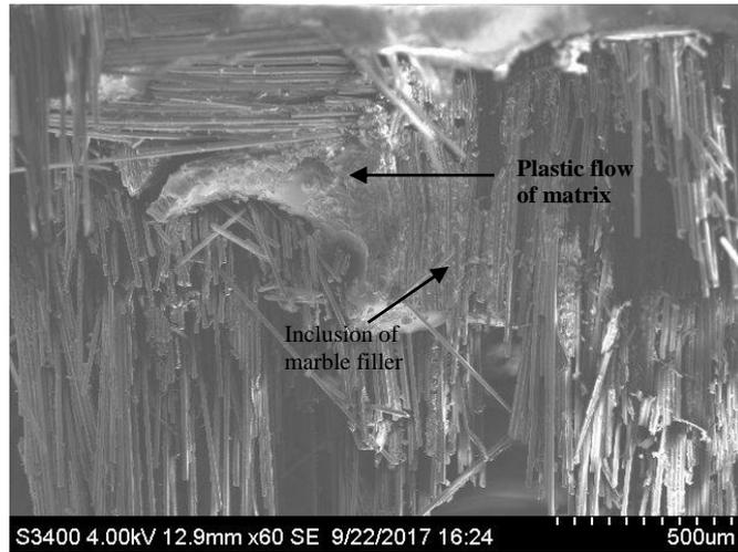
**Fig.8.c - Micrograph of EGM2 sample after impact test**
