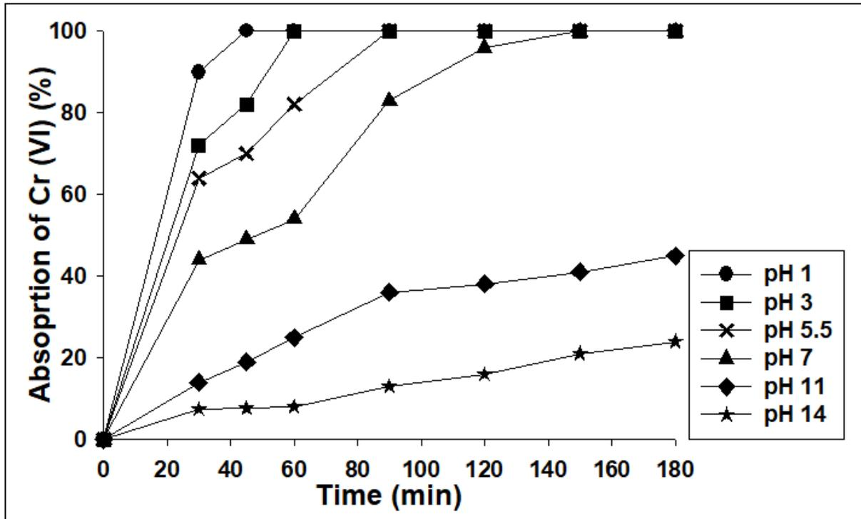
Figure 1: Effect of solution pH on the Cr (VI) removal rate with PVA-alginate beads.
