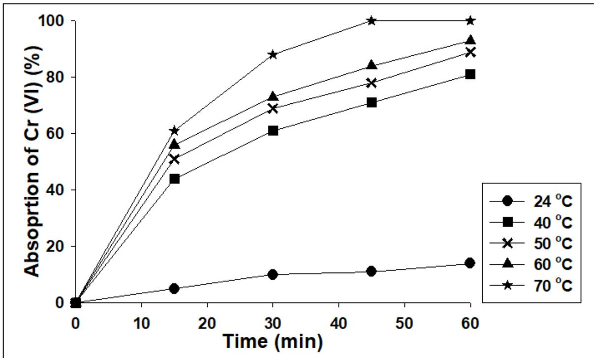
Figure 2: Effect of temperature on the Cr (VI) removal rate with PVA-alginate beads.
