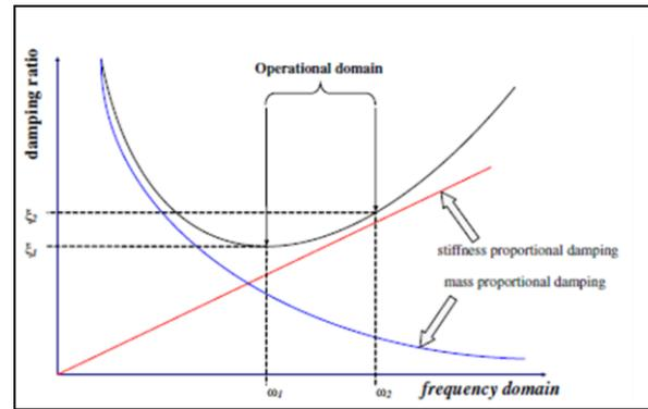
Fig. 1: Relationship of Mass and Stiffness Proportional Term with Damping Ratio and Natural Frequencies [10].
