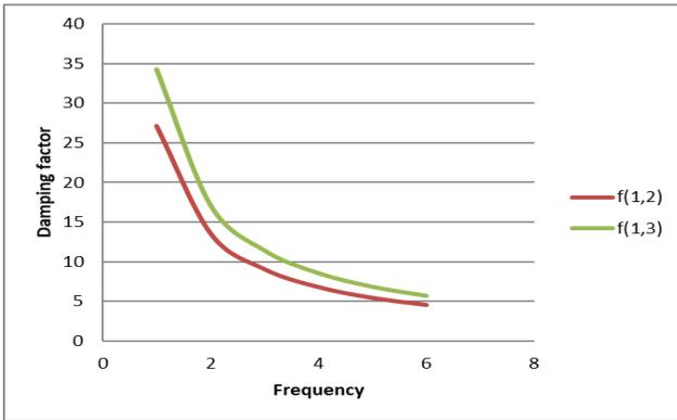
Fig. 4: Graph from First Mode of Damping Ratio for Steel Plate
