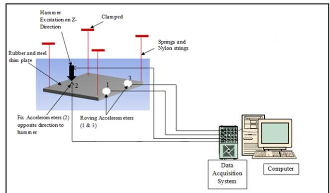
Fig. 3: Full Diagram of Steel and Rubber Plates Testing
