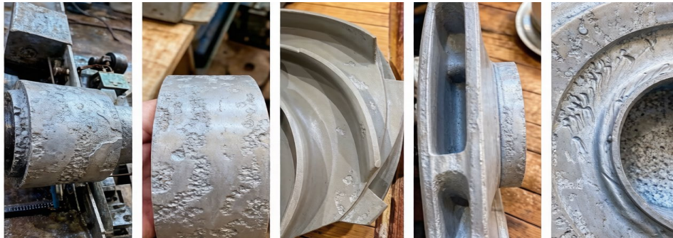
Fig. 3 Common cavitation erosion positions of pump body
