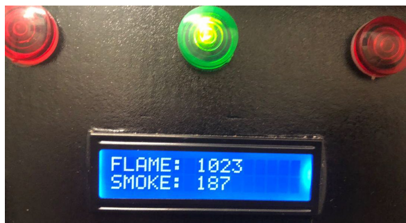
(a) Real-time smoke and flame sensor readings displayed on the LCD
