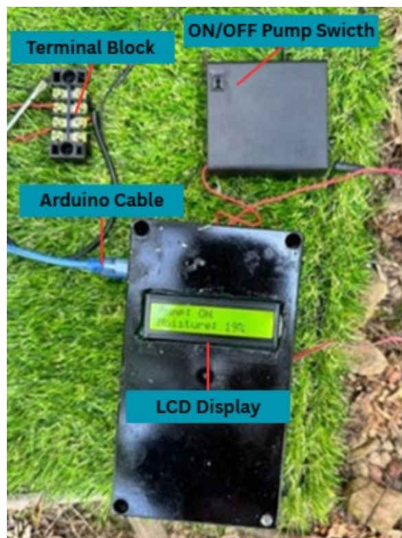
Fig. 8 The LCD screen indicates pump activation by displaying "ON"
