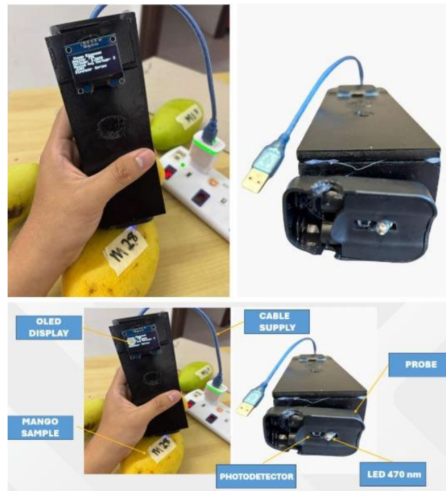
Fig. 6 Images of the developed prototype of a handheld optical device showing how it is used for detecting mango ripeness. Main components are labelled accordingly
