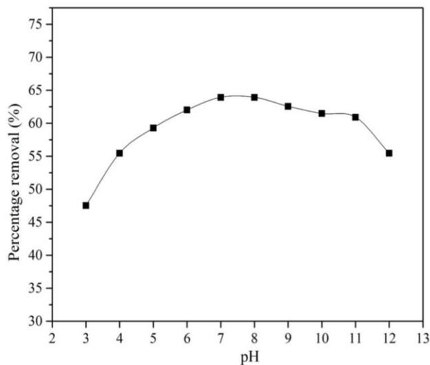
Fig. 3 Effect of pH on adsorption of colour
