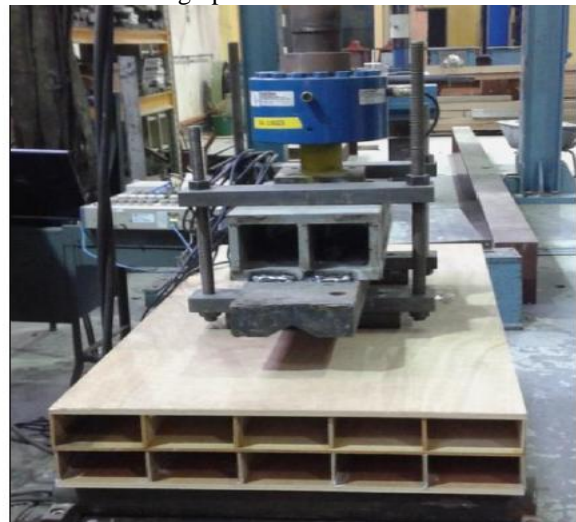
Fig 10 Flexural test arrangement
