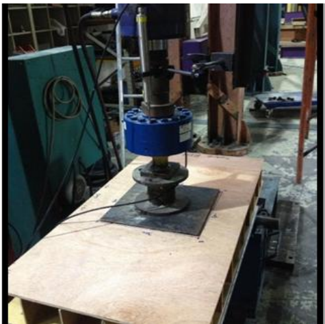
Fig. 12 Complete setup arrangement for the punching shear test
