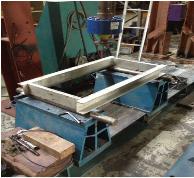
Fig. 11 Metal rectangular support for the honeycomb sandwich panel
