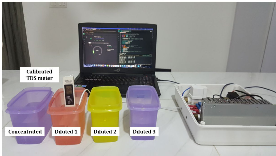
Fig. 5 Accuracy test of the TDS sensor using different ppm solutions
