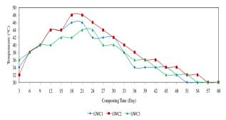
Fig. 2 The changes of temperature over composting period
