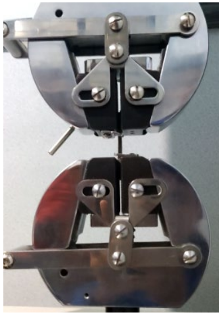
Fig. 3 Real-time UTM testing setup as per ASTM D638 type V
