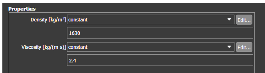
Fig. 1 Input parameters for density and viscosity in Ansys Fluent
