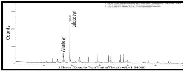
Fig. 5 Topas semi-quantitative analysis of precipitates formed from addition of calcium chloride (Crystal 74.4% and 25.6%).
