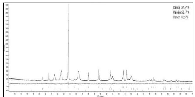
Fig. 4 Diffractogram of precipitates formed from addition of calcium chloride (Calcite 37.57%, Vaterite 56.17% and 6.26%)
