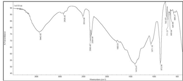
Fig. 2 FTIR spectra of precipitates formed from addition of calcium chloride into fermentation supernatant.
