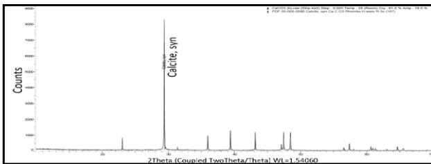
Fig. 7 Topas semi-quantitative analysis of precipitates formed from addition of calcium nitrate tetrahydrate (Crystal 81% and amp 19%)
