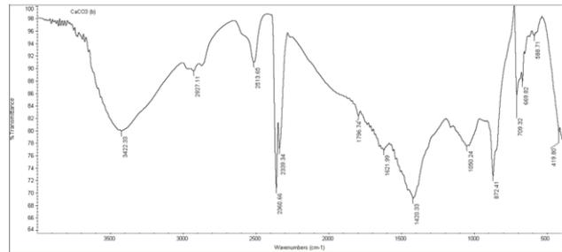
Fig. 3 FTIR spectra of precipitates formed from addition of calcium nitrate tetrahydrate into fermentation supernatant
