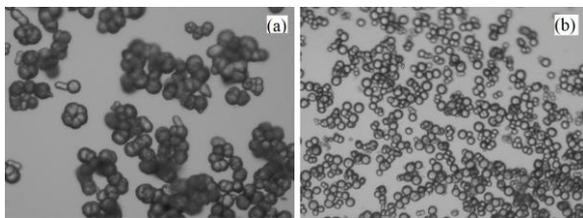
Fig. 1 Calcium carbonate produced from addition of calcium nitrate tetrahydrate (a) and calcium chloride (b) under microscope (100X)
