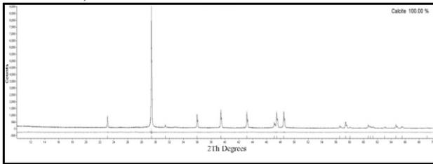
Fig. 6 Diffractogram of precipitates formed from addition of calcium nitrate tetrahydrate (Calcite 100%)
