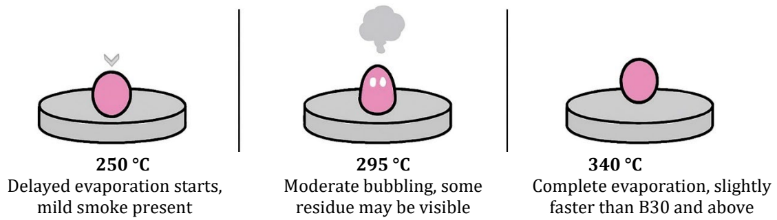
Fig. 4 B20 droplet evaporation behaviour
