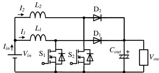
Fig. 2 - 2-phase interleaved DC-DC boost converter (IBC)
