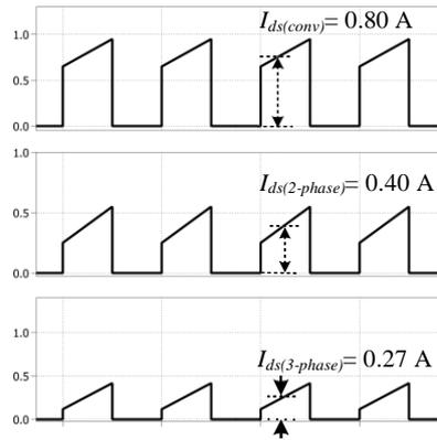
**Fig. 9 - Simulation result of current stress on switching device (MOSFET)**
