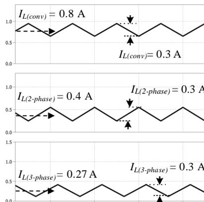
**Fig. 8 - Simulation result of current stress on inductor**
