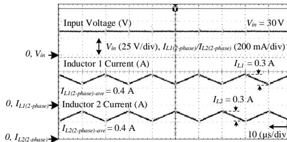
**Fig. 11 - Input voltage and the current stress/ripple of the 2-phase IBC**
