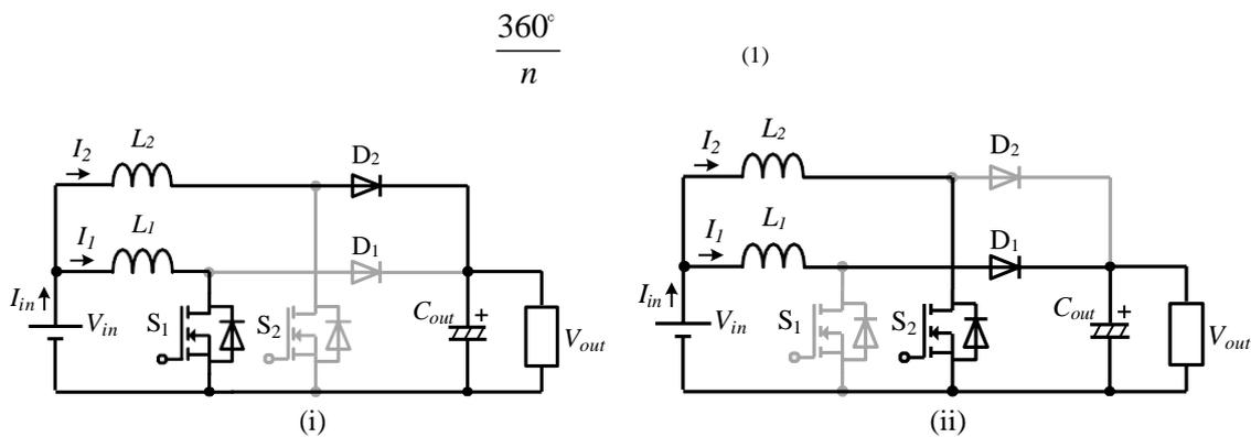
Fig. 3 – Operation mode of 2-phase IBC (i) Mode 1 (ii) Mode 2
