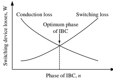
**Fig. 7 - Losses against phase number of IBC**
