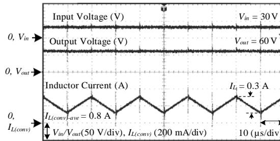
**Fig. 10 - Input voltage, output voltage and inductor current stress/ripple of the conventional DC-DC boost converter**
