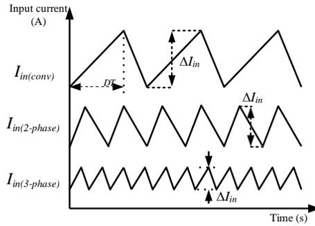
Fig. 5 - Input current ripple reduction of multiphase IBC
