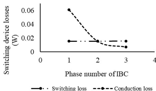
**Fig. 13 - Switching device losses in MOSFET against phase number of IBC**
