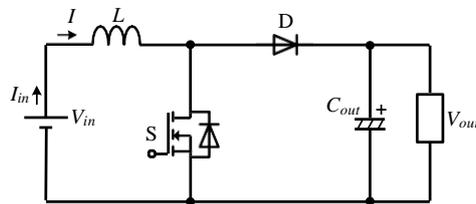
Fig. 1 - Conventional DC-DC boost converter
