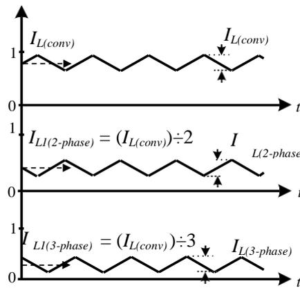
Fig. 6 - Reduction of current stress in conventional DC-DC boost converter, 2-phase IBC and 3-phase IBC
