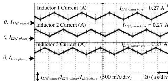
**Fig. 12 - The current stress/ripple of the 3-phase IBC**
