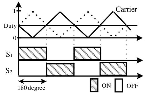
Fig. 4 - 180-degree phase shifted PWM of 2-phase IBC
