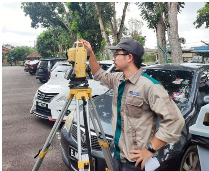
Fig. 2 TOPCON total station
