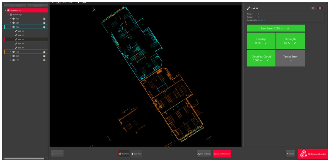
Fig. 10 The optimization of the link between setup 1 (E) and setup 2 (C) resulted in an overlapping percentage of 36%. The optimized link is denoted as having 66% strength, with no errors detected
