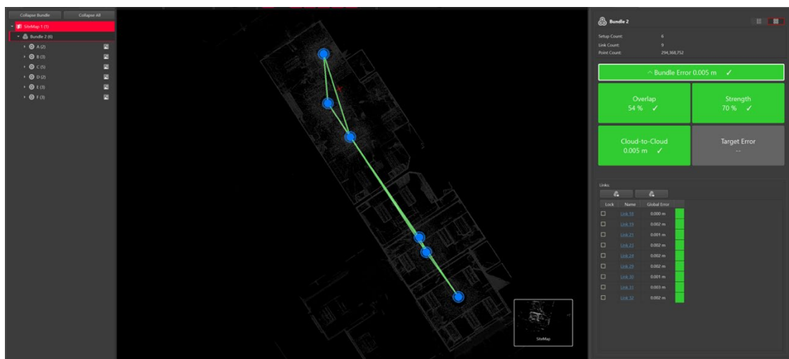
Fig. 9 The TLS setup configurations, spanning from setup 1 (A) to setup 6 (F), demonstrate an overall overlapping percentage of 54% within bundle links, along with an overall strength of 70%, with no errors detected
